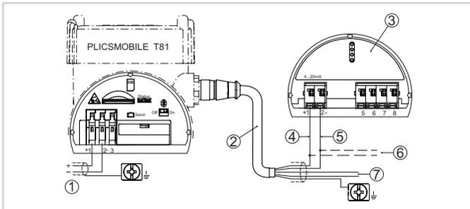
Connection of the voltage supply in the electronics housing
