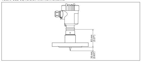
Fig. 44: VEGAPULS 66, version with horn antenna
