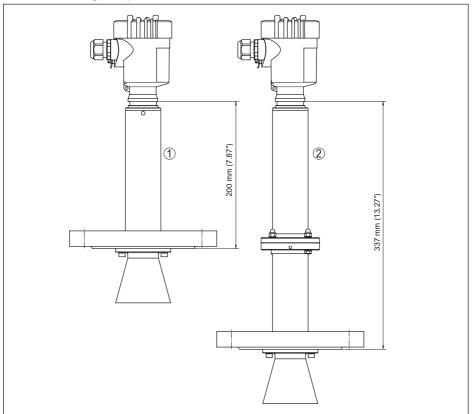
Fig. 45: VEGAPULS 66, high temperature version
