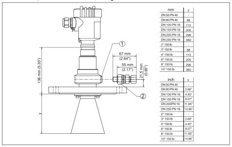
Fig. 43: VEGAPULS 66, standard version with rinsing air connection
