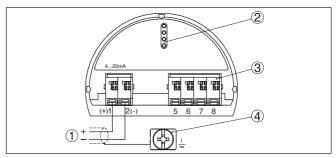
Fig. 16: Electronics and connection compartment - single chamber housing
