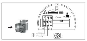
Fig. 19: Connection compartment - Radio module PLICSMOBILE 81
