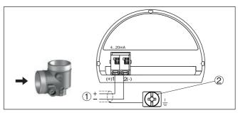
Fig. 21: Connection compartment - Ex-d-ia double chamber housing
