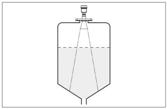
Fig. 4: Vessel with conical bottom
