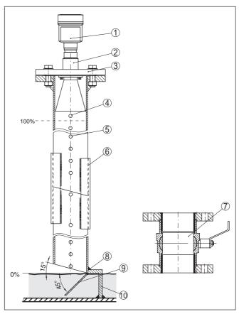
Fig. 12: Configuration surge pipe VEGAPULS 66
