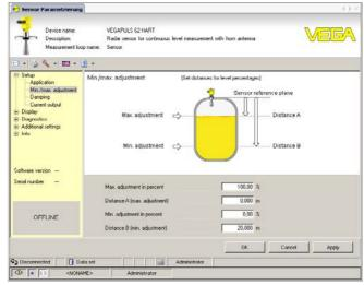
Fig. 33: Example of a DTM view
