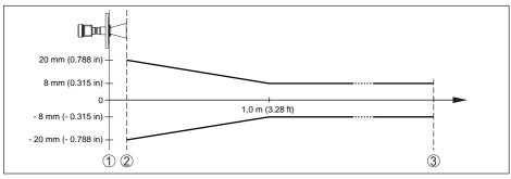
Fig. 36: Deviation under reference conditions
