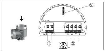
Fig. 20: Electronics compartment - Ex-d-ia double chamber housing
