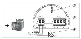
Fig. 18: Connection compartment - double chamber housing
