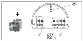
Fig. 17: Electronics compartment - double chamber housing
