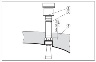
Fig. 11: Mounting the instrument on insulated vessels.
