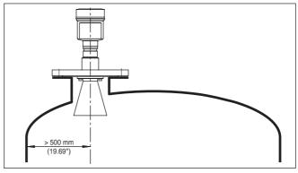
Fig. 3: Mounting on round vessel tops
