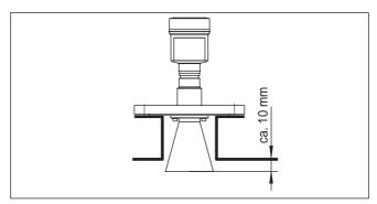
Fig. 6: Recommended socket mounting
