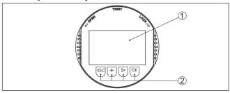
Fig. 28: Display and adjustment elements
