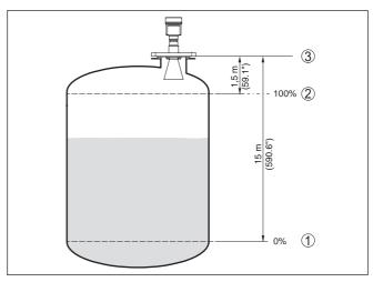
Fig. 30: Parameterisation example, Min./max. adjustment
