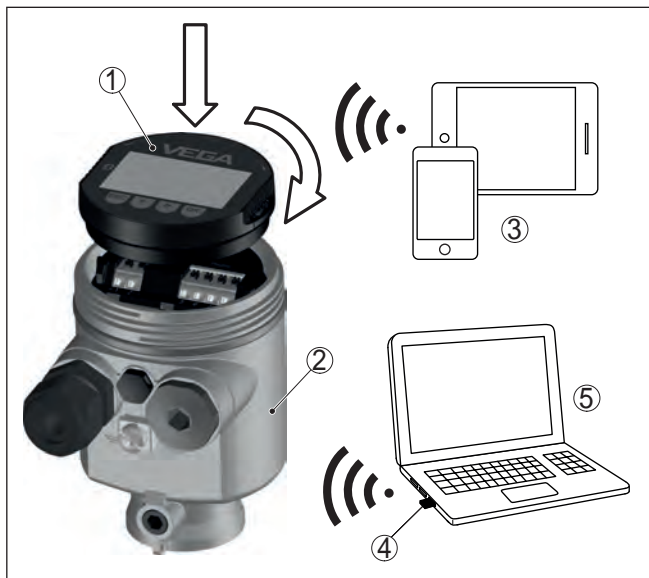
Fig. 2: Wireless connection to standard operating devices
