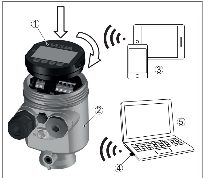
Fig. 2: Wireless connection to standard operating devices
