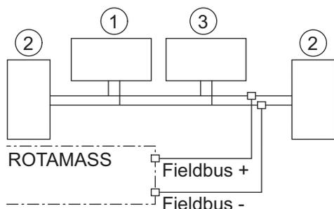
Fig. 43: FOUNDATION Fieldbus connection
