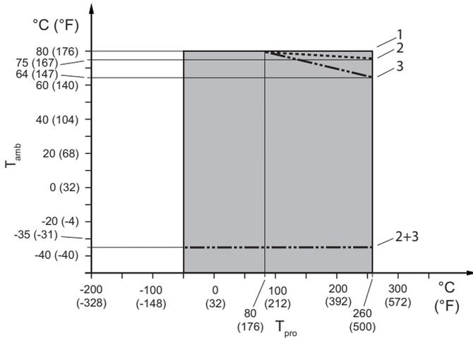
Fig. 19: Allowed process fluid and ambient temperatures
