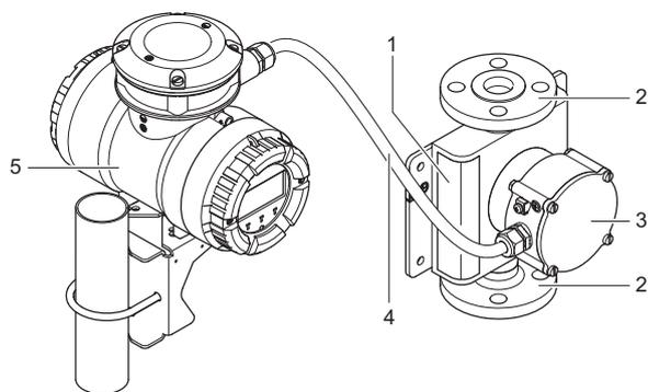
Fig. 2: Configuration of the Rotamass remote type
