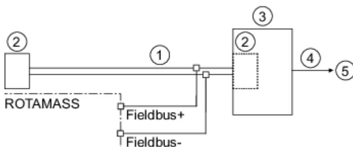
Fig. 42: PROFIBUS PA connection
