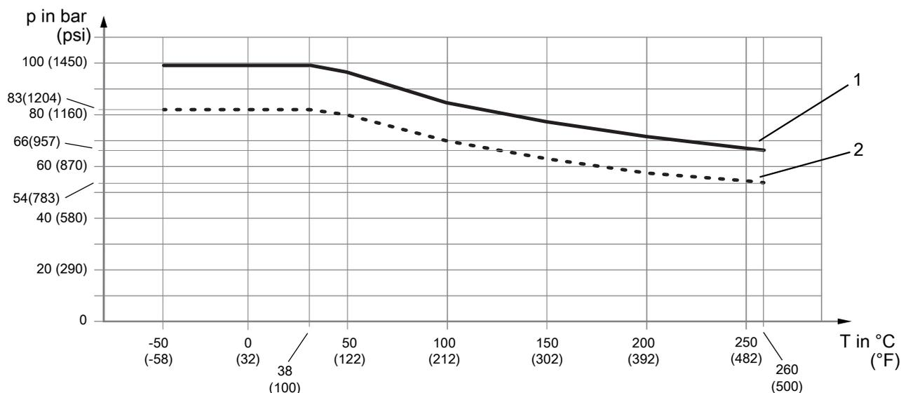
Fig. 9: Allowed process pressure as a function of process connection temperature
