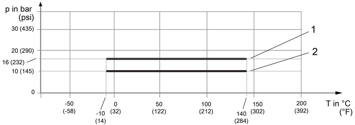
Fig. 13: Allowed process pressure as a function of process fluid temperature
