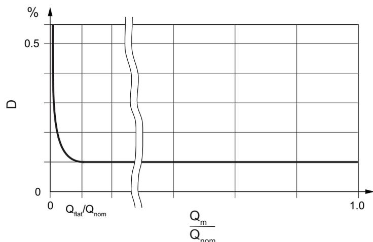
Fig. 4: Schematic dependency of the maximum deviation on the mass flow
