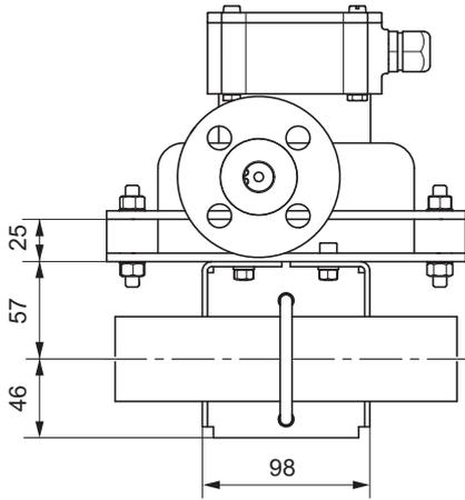
Fig. 23: Dimensions in mm: fixing device option PD for Nano
