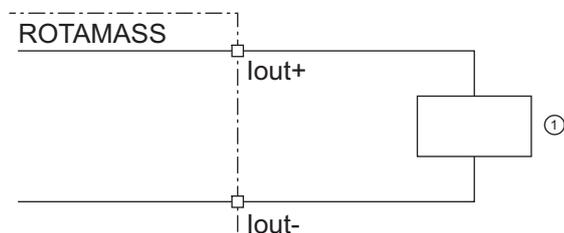
Fig. 26: Active current output connection *I<sub>out</sub>* HART
