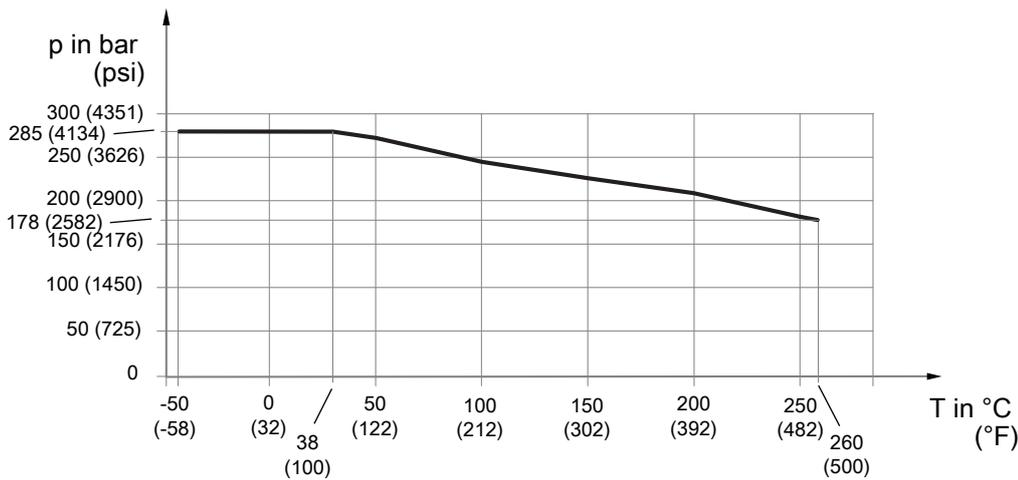
Fig. 15: Allowed process pressure as a function of process fluid temperature
