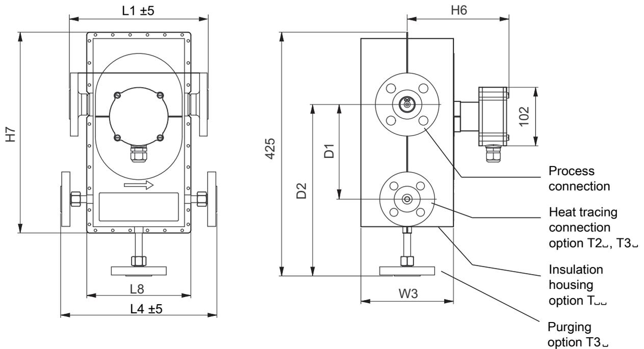
Fig. 22: Dimensions in mm: version with insulation housing for meter sizes Intense 34, 36 and 38 only
