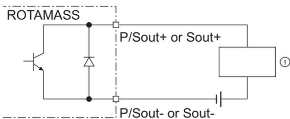
Fig. 38: Passive status output connection P/Sout or Sout
