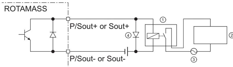
Fig. 39: Passive status output connection *P/Sout* or *Sout* for solenoid valve circuit
