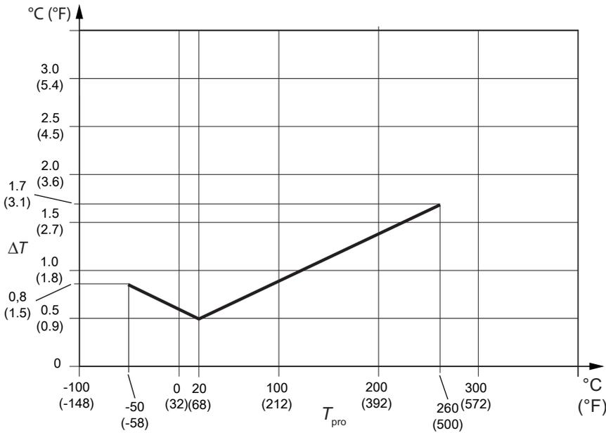
Fig. 5: Temperature accuracy
