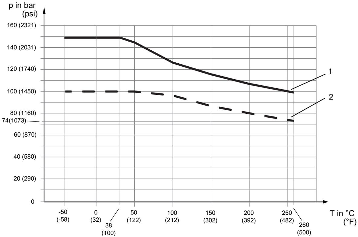
Fig. 10: Allowed process pressure as a function of process connection temperature
