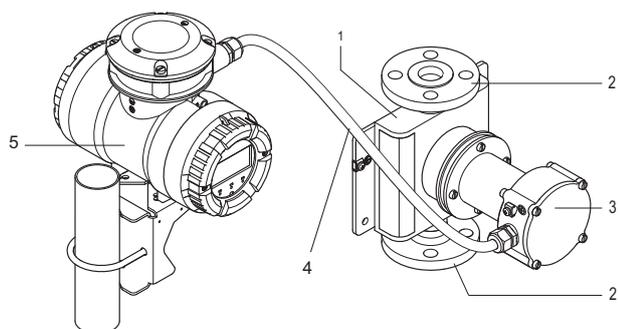
Fig. 3: Configuration of the Rotamass remote type - long neck
