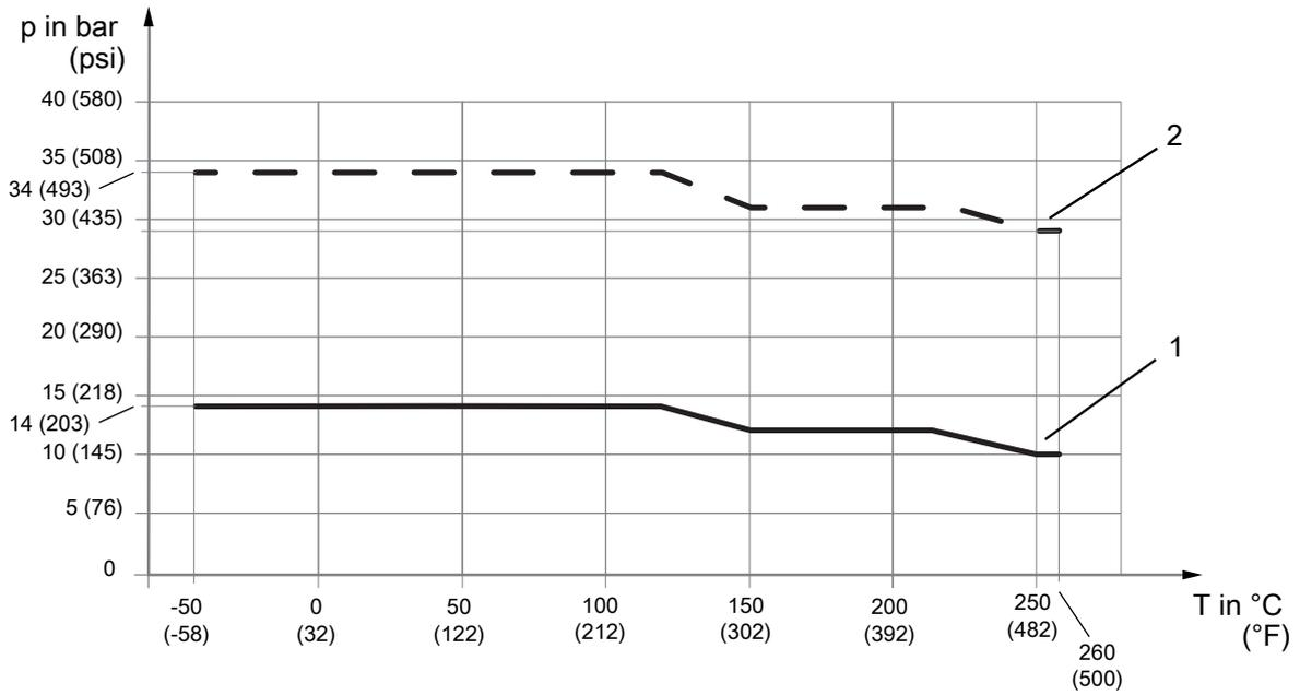
Fig. 12: Allowed process pressure as a function of process connection temperature
