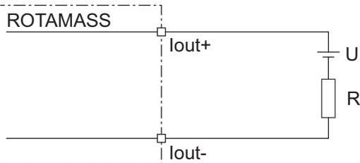
Fig. 28: Passive current output connection *lout*
