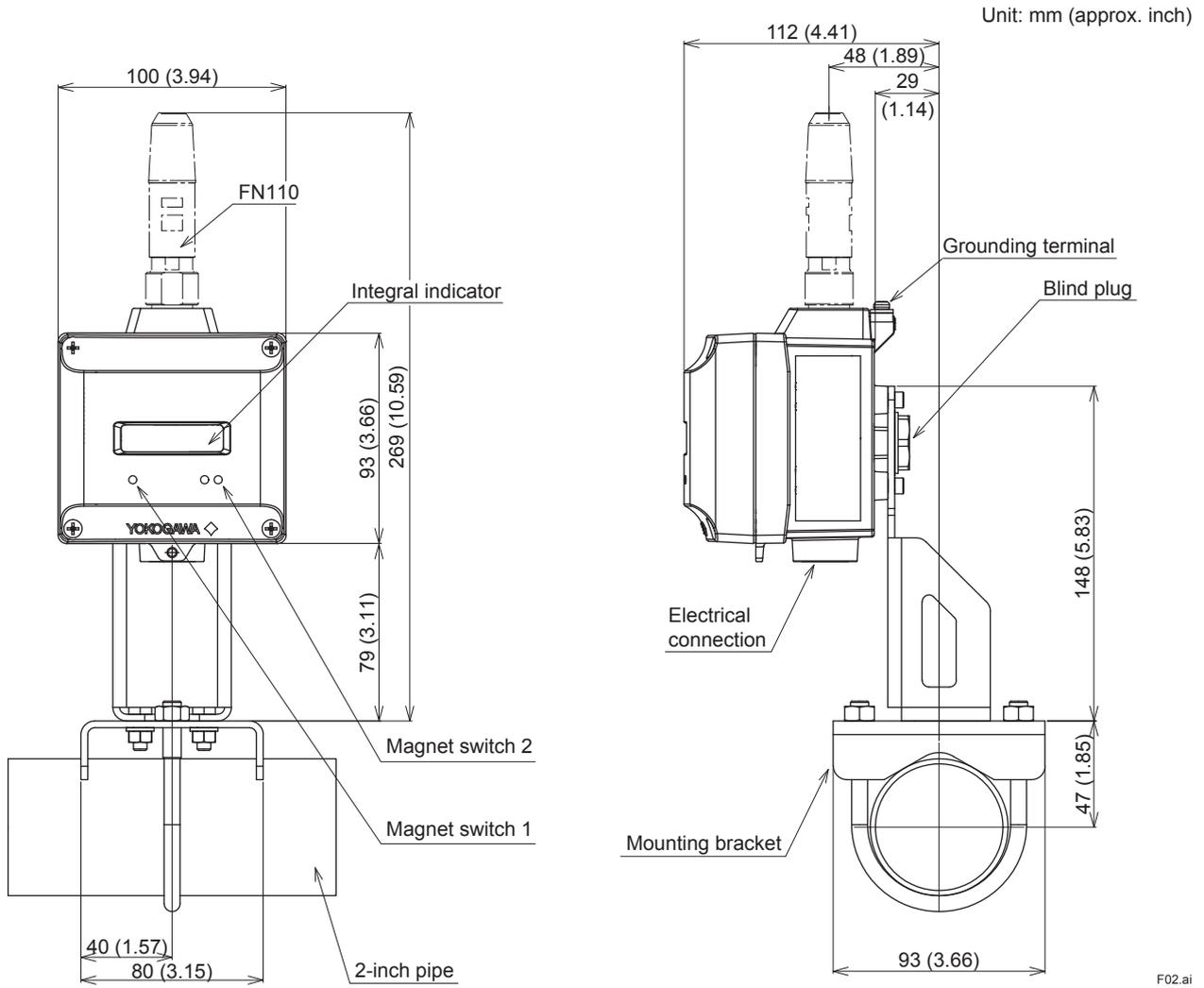
□ 2-inch pipe mounting (for vertical piping) (Protocol code: J, M)
