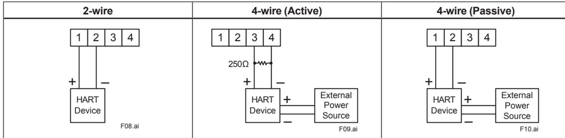
\* Connect the FN310 and HART devices directly.
