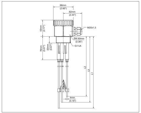
Fig. 7: Conductive multiple rod electrode EL 4
