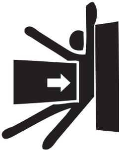
Do not stand or place hand in front of valve discharge flange if valve is under pressure.
