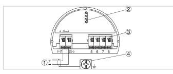
Electronics and terminal compartment, single chamber housing
