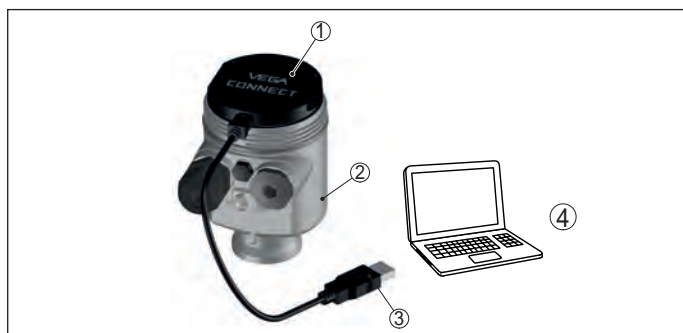
Fig. 23: Connection of the PC via VEGACONNECT and USB
