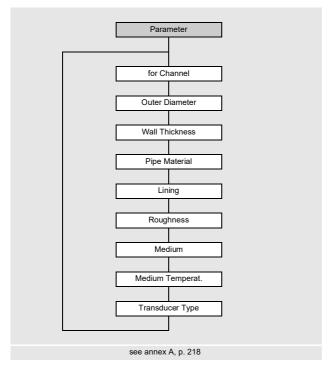
The pipe and fluid parameters are entered for the selected measuring point. The parameter ranges are limited by the technical characteristics of the transducers and the transmitter.
