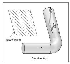
The sound beam plane is selected in an angle of 90° ± 45° to the elbow plane.
