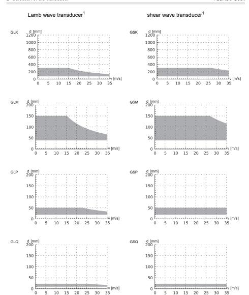
1 inner pipe diameter and max. flow velocity for a typical application with natural gas, nitrogen, oxygen in reflection arrangement with 2 sound paths (Lamb wave transducers)/1 sound path (shear wave transducers)
