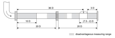
Considering flow profile and influence of noise, the measuring point can be selected in the area 3...(7.5 - 2) D on the right side of pipe segment 2 (with max. distance from the elbow).
