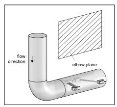
The sound beam plan is selected in an angle of 90° to the elbow plane. The elbow is upstream of the measuring point.
