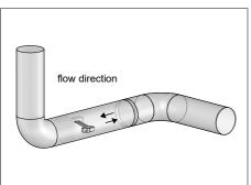
The sound beam plane is selected according to the nearest elbow (horizontal or vertical, depending on the pipe orientation, see above).
