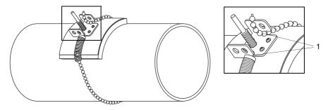
1 - slots on the upper side of the temperature probe
