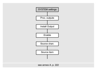
If the transmitter is equipped with outputs, they have to be installed and activated before they can be used:
