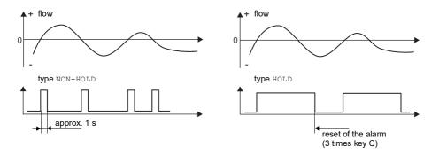
When adjusting to changed measurement conditions e.g, a substantial increase of the fluid temperature, the alarm will not be switched. Alarm outputs with the switching condition <code>OFF</code> will be set automatically to the switching function <code>NO Cont</code>.
