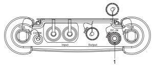
1 - power supply unit/battery charging unit
