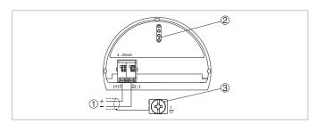
Electronics and terminal compartment, single chamber housing
