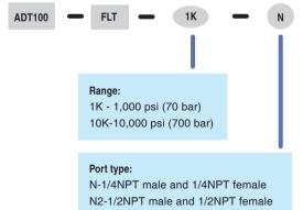
N2-1/2NPT male and 1/2NPT female B-1/4BSP male and 1/4BSP female B2-1/2BSP male and 1/2BSP female M-M20x1.5 male and M20x1.5 female
