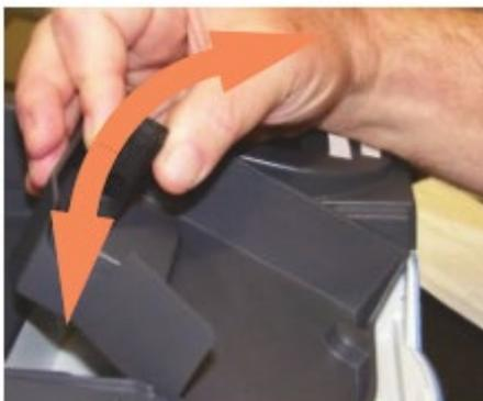
Insertion – allow front magnet to engage. Lower cell holder into place, allowing back magnet to guide and engage
