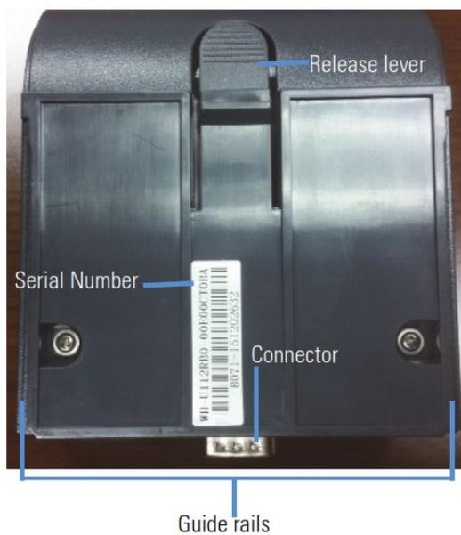
5. Push the printer forward until the connectors are fully connected. You will hear a snap when the connectors have engaged properly.
