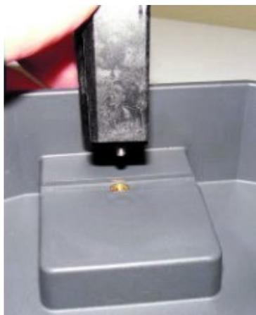
Loosen the captive screw and the base of the cell holder to remove it. Attach a new sample holder in the same way.
