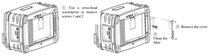
Figure 8-4 Disassembly and assembly of the air filter
