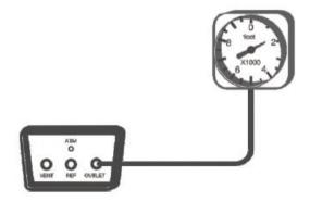
Figure 5-10 Calibration of the barometric altimeter
