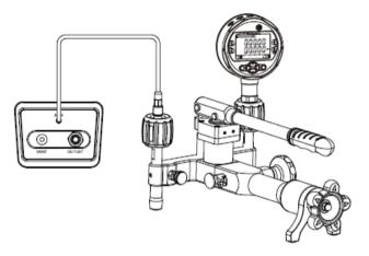
Figure 4-1 Calibrate an barometric pressure module
