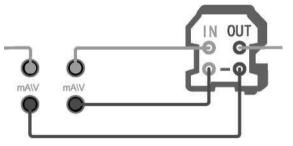
Figure 5-3 Calibration of the signal isolator
