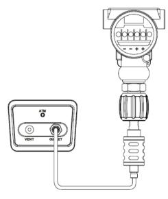
Figure 3-3 Gauge pressure outlet
