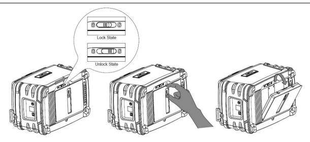
Figure 2-3 Battery installation
