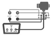
Figure 5-2 Calibration of the pressure sensor
