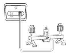
Figure 2-5 Gauge pressure connection
