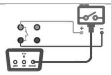
Figure 3-16 Calibration of a pressure switch
