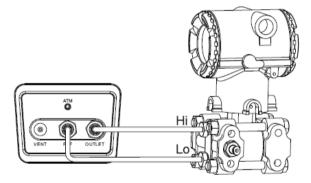
Figure 3-2 Differential pressure outlet
