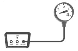
Figure 3-12 Calibration of a pressure gauge
