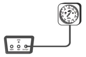
Figure 5-9 Calibration of the aneroid barometer
