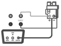
Figure 3-17 Calibration of an I/P converter
