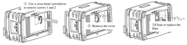
Figure 8-1 Disassembly of the suction filter
