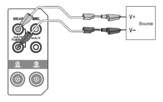
Figure 3-6 Voltage measurement
