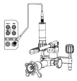
Figure 3-11 Connection of the external module
