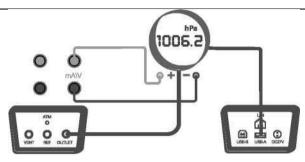
Figure 5-7 Calibration of the VAISALA digital barometer
