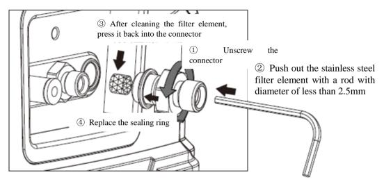
Figure 8-3 Disassembly of differential pressure connector
