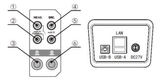
Figure 2-2 Electrical and signal port
