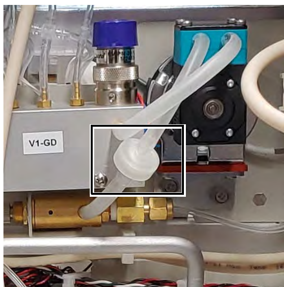
Figure 84: Replacing the Disc Filter
