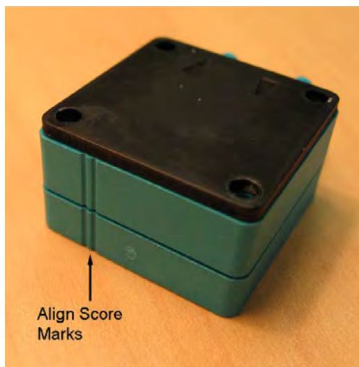
Figure 88: Aligning the Pump Head Plates
