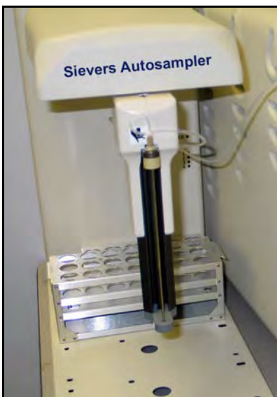
Figure 18: Lowering the Sievers Autosampler Arm
