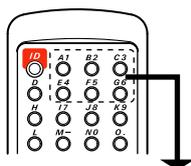
The character string switches in the following order each time the key is pressed. The display switches in a cyclic pattern.
