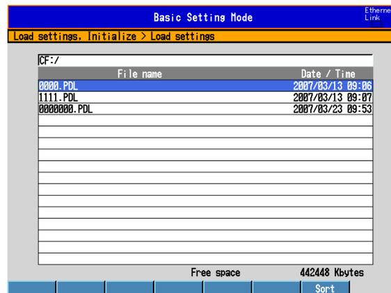
2. Use **DISP/ENTER** and **arrow keys** to select the setup file to be loaded.
