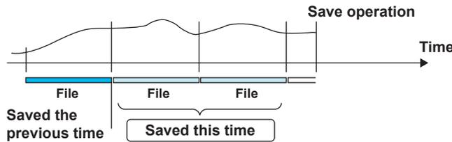
When using manual save, it is important that you save the data in the internal memory to the external storage medium before the data is overwritten. Determine the usage condition of the internal memory and save the data to the external storage medium at appropriate times.
