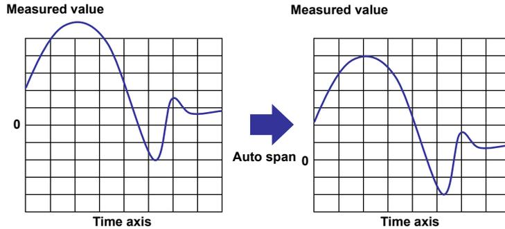
When the maximum or minimum values are within the set display span
