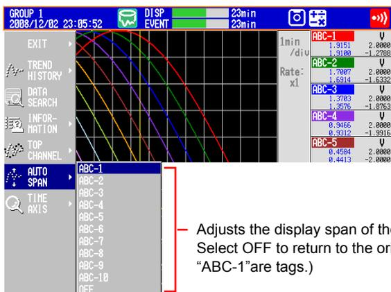
Adjusts the display span of the selected channel. Select OFF to return to the original span. (List items like “ABC-1” are tags.)
