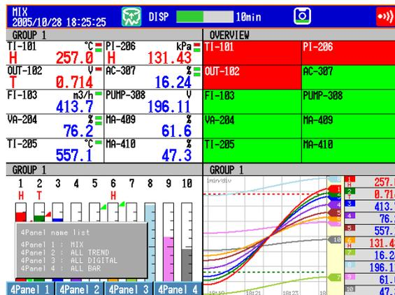
3. Press any of the **4Panel 1** to **4panel 4** soft keys to display a window used to enter the display name.
