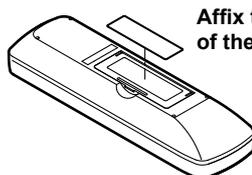
Affix the ID number label on the battery cover of the remote control terminal.
