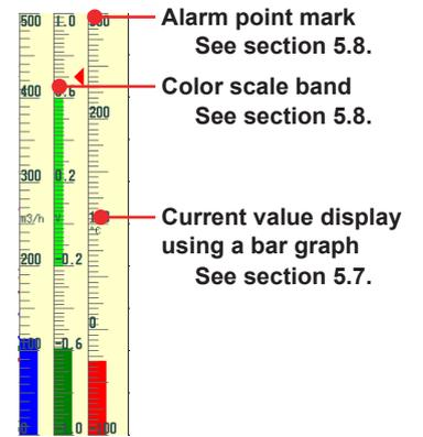
Displays the maximum and minimum values of the data sampled within the time corresponding to 1 dot.
