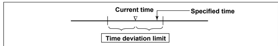
When the time deviation between the time on the DX and the specified time is within  $\pm$ (the value specified here), the time on the DX is gradually corrected. Otherwise, the clock is corrected immediately. Note that time is not corrected on DXs with the Advanced security function (/AS1 option) when the specified time is over the time deviation limit. (Firmware version numbers 4.11 and later)
