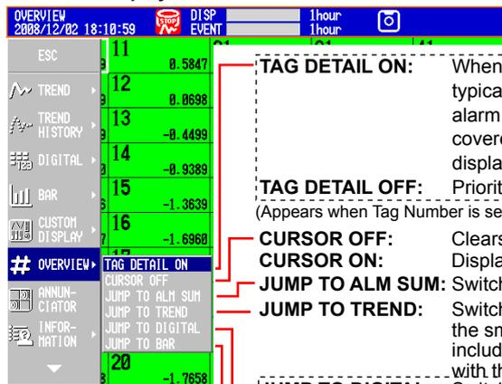
**TAG DETAIL ON:** When a tag does not fit into the typical tag display space, the alarm and measured values are covered so that the tag can be displayed completely.
