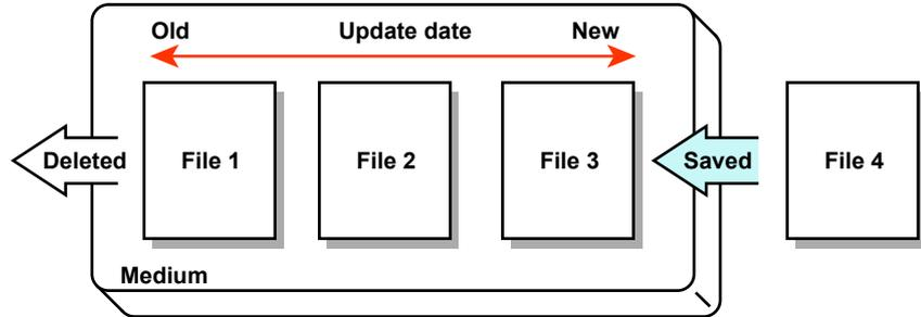
If not enough free space is available when saving a new data file to the CF card, files are deleted in order from the oldest data update date/time to save the new file. This operation is referred to as FIFO (First In First Out).
