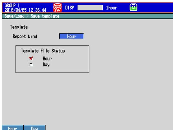
Under Template File Status, the check boxes of the template files that are stored in the internal memory are selected.
