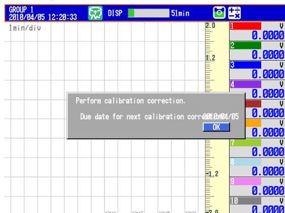
The calibration notification screen only appears over operation screens. It will continue to appear until you perform calibration (Finish Calibration).
