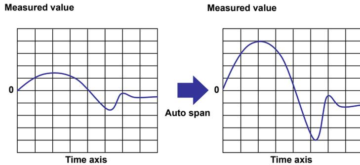
If the maximum or minimum data value falls outside the maximum selectable display span, the DX adjusts the display span to the maximum or minimum possible value. The DX responds in the same way when it encounters overflow data.
