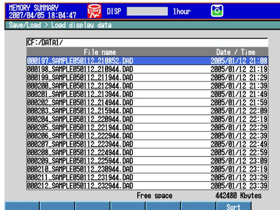
3. Press the **arrow keys** to select a file, and press **DISP/ENTER**. The file is loaded, and the waveform is displayed in the historical trend.
