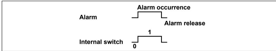
The internal switches can be used events of the event action function (see section 1.6). In addition, the internal switches can be written in calculation expressions of computation channels (/M1 or /PM1 option).
