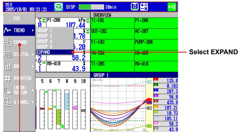
This **EXPAND** is not shown under the initial conditions. To show, operate as follows:
