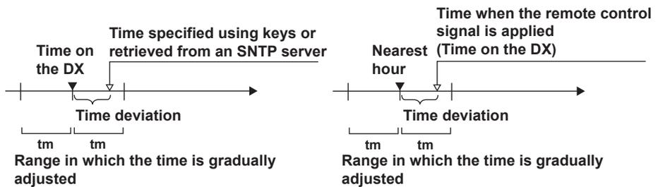
Example: When changing the time to 12 hours 55 minutes 35 seconds when the internal clock is 12 hours 55 minutes 32 seconds
