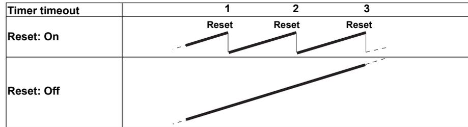
When reset is On, the sum value is calculated over each interval. When set to Off, the sum value from computation start is calculated.
