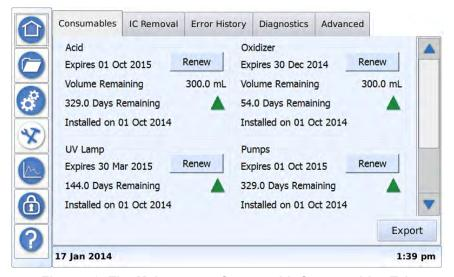
Figure 53: The Maintenance Screen with Consumables Tab
