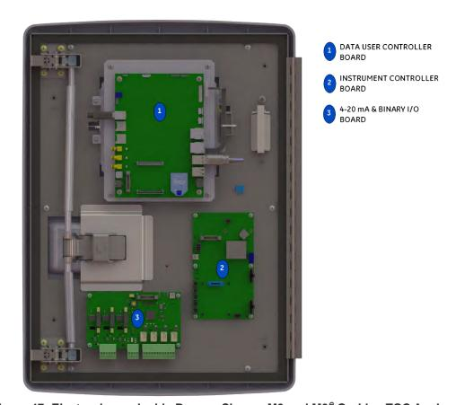
Figure 47: Electronics on Inside Door — Sievers M9 and M9<sup>e</sup> On-Line TOC Analyzers
