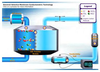
Figure 4: Sample Flow through the CO<sub>2</sub> Transfer Module
