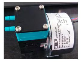
Figure 68: ICR Pump and Diaphragm Housing
