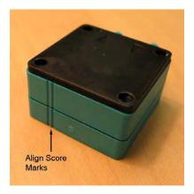
Figure 70: Aligning the Pump Plates
