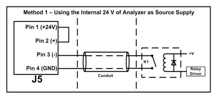
Figure 15: Wiring Option for Binary Input — Using Analyzer's Internal Supply
