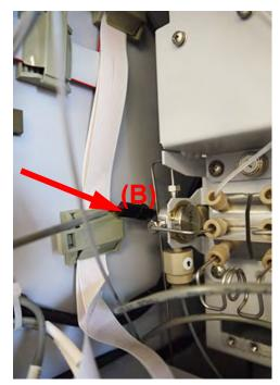
Figure 82: Jumper Cable Connection for ICR Pump
