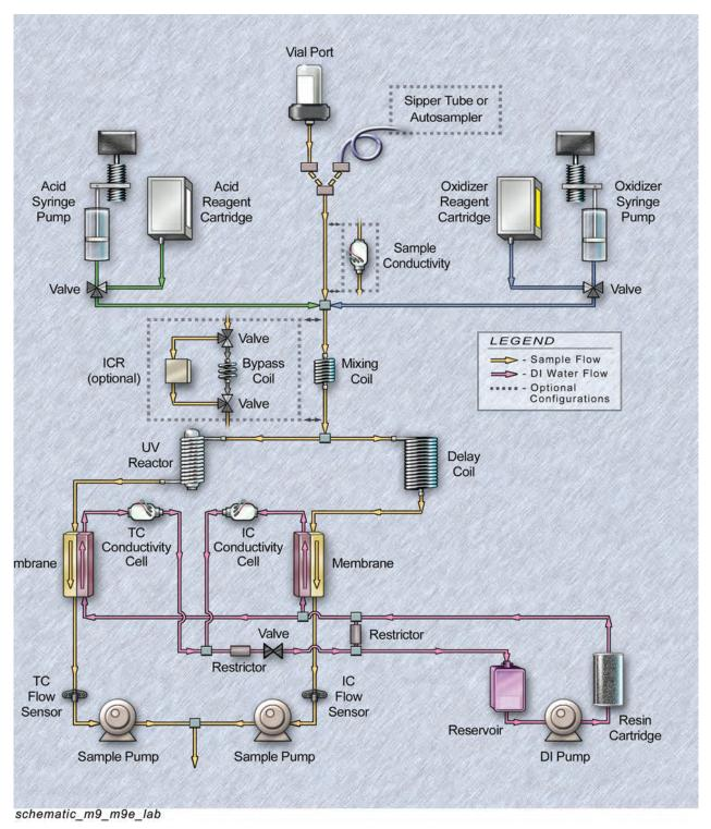
Figure 3: Sievers M9 and M9<sup>e</sup> TOC Analyzers Schematic — Laboratory Model Samples are introduced to the Analyzer as follows:
