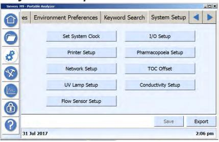
Figure 33: System Setup Tab - M9 TOC Analyzers
