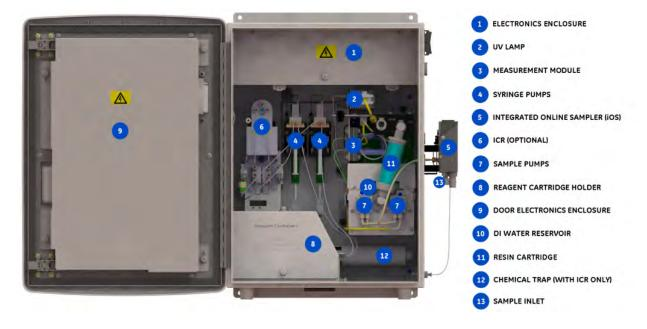
Figure 45: Interior Overview — Sievers M9 and M9<sup>e</sup> On-Line TOC Analyzers
