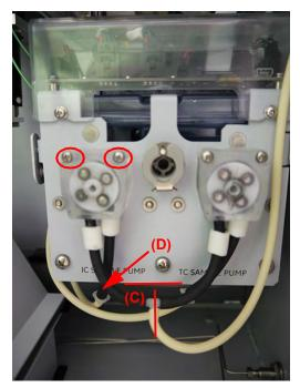
Figure 58: Sample Pump Heads and Tubing — IC Side
