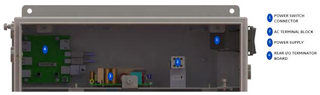
Figure 46: Electronics Enclosure (Top Shelf) — M9 and M9<sup>e</sup> On-Line Analyzers
