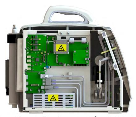
Figure 51: Electronics Side — Sievers M9 and M9<sup>e</sup> Portable TOC Analyzers
