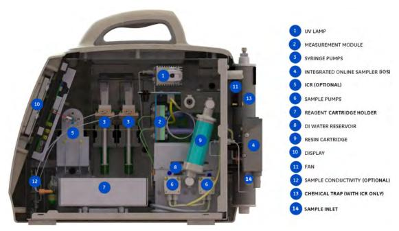
Figure 50: Fluidics Side — Sievers M9 and M9<sup>e</sup> Portable TOC Analyzers
