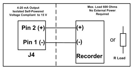
Figure 14: Wiring 4-20 mA Connections
