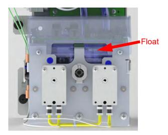
Figure 12: DI Reservoir Level with Float
