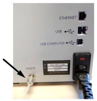
Figure 21: Waste Outlet Fitting — Laboratory TOC Analyzer
