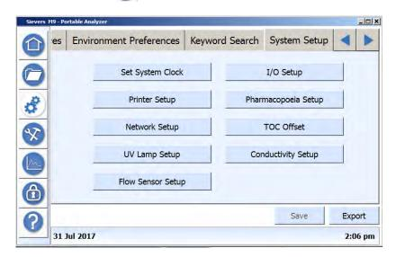
Figure 95: System Setup Tab - M9 TOC Analyzer
