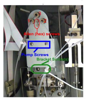
Figure 81: Tubing Connections and Screw Placement
