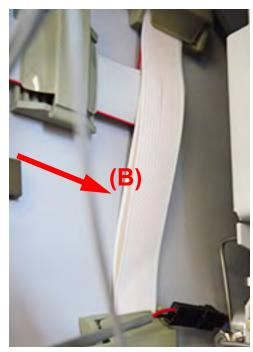
Figure 75: Jumper Cable Connection for ICR Pump
