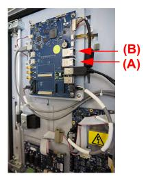
Figure 99: Internal Ethernet Ports — On-Line TOC Analyzer
