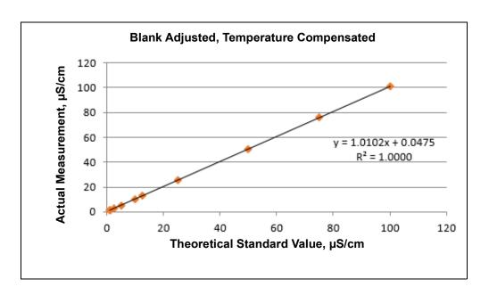
Figure 5: Linearity of M9/M9<sup>e</sup> TOC Analyzers' Conductivity Measurement Conducting validations can be performed for two purposes:
