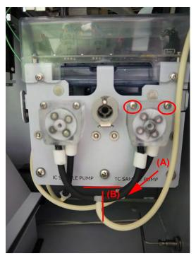
Figure 57: Sample Pump Heads and Tubing — TC Side
