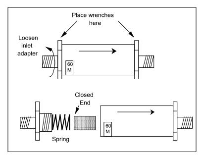
Figure 60: Replacing the In-Line Filter Element
