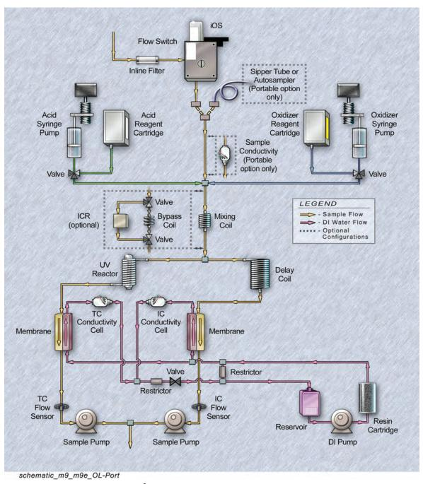
Figure 2: Sievers M9 and M9<sup>e</sup> TOC Analyzers Schematic — On-Line and Portable Models
