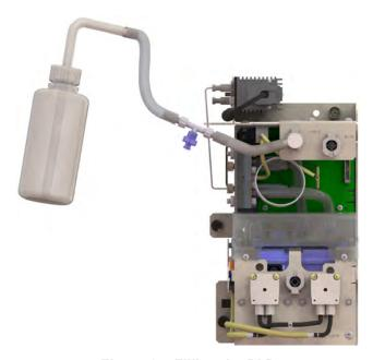
Figure 84: Filling the DI Pump
