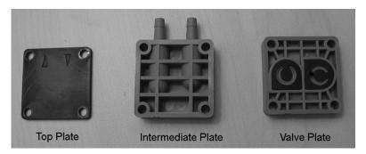
Figure 78: ICR Pump Plates
