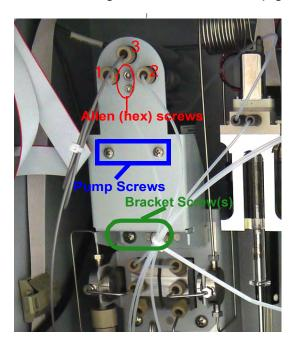
Figure 72: Tubing Connections and Screw Placement
