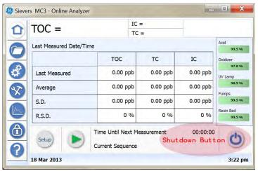
Figure 28: The Shut Down Button
