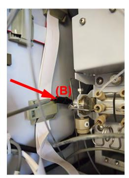
Figure 64: Jumper Cable Connection for ICR Pump
