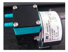
Figure 80: Correct Orientation — Pump Head and Motor
