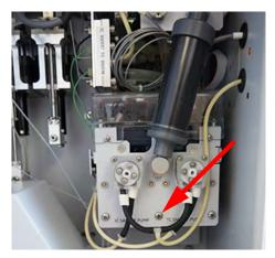
Figure 91: TC/IC Y-Connector
