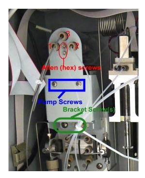
Figure 67: ICR Bracket - Removing Tubing Connections and Screws
