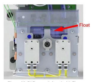
Figure 85: DI Reservoir Level with Float
