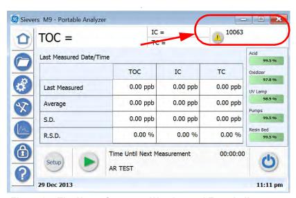
Figure 27: The Home Screen — Warning and Error Indicator
