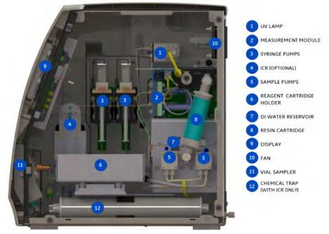
Figure 48: Fluidics Side — Sievers M9 and M9<sup>e</sup> Laboratory TOC Analyzers
