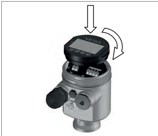
Fig. 34: Installing the display and adjustment module in the electronics compartment of the single chamber housing
