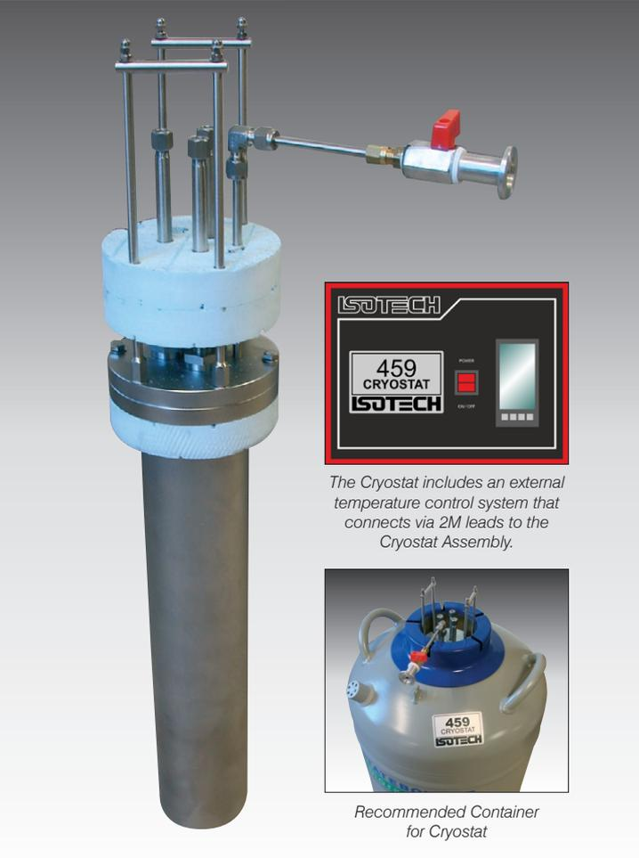
The Cryostat includes an external temperature control system that connects via 2M leads to the Cryostat Assembly.
