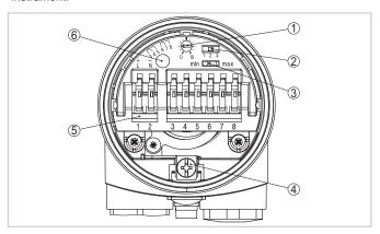
Oscillator with relay output
