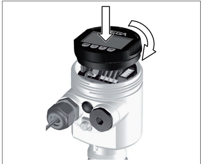
Fig. 16: Insert display and adjustment module in the single chamber housing
