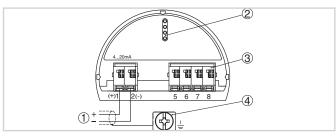
Electronics and terminal compartment, single chamber housing
