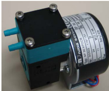
Figure 71: Correct Orientation — Pump Head and Motor
