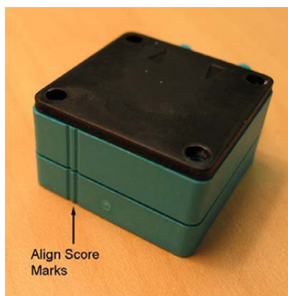
Figure 79: Aligning the Pump Plates
