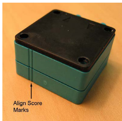
Figure 70: Aligning the Pump Plates
