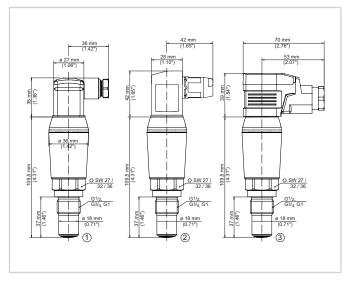
VEGAPOINT 24, standard version - thread with valve plugs acc. to ISO 4400
