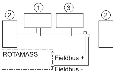
Fig. 37: FOUNDATION Fieldbus connection
