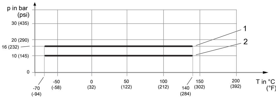
Fig. 11: Allowed process pressure as a function of process connection temperature
