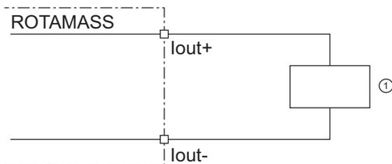
Fig. 20: Active current output connection *lout* HART
