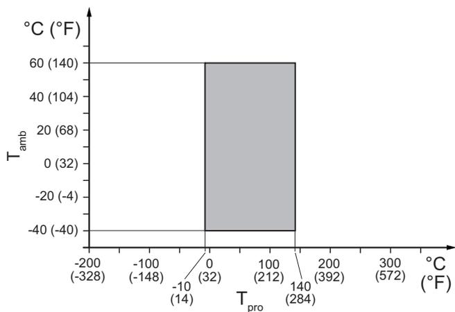
Fig. 13: Allowed process fluid and ambient temperatures, integral type for process connection type HS4 and HS8
