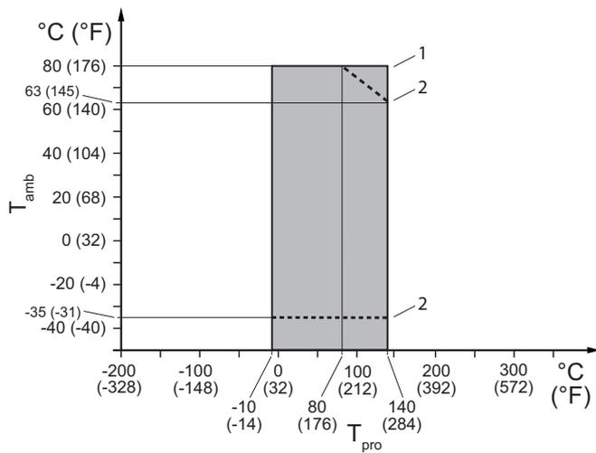
Fig. 15: Allowed process fluid and ambient temperatures, remote type for process connection type HS4 and HS8
