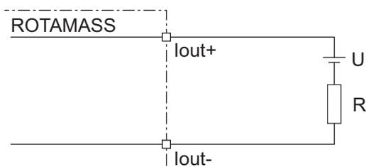
Fig. 22: Passive current output connection *lout*
