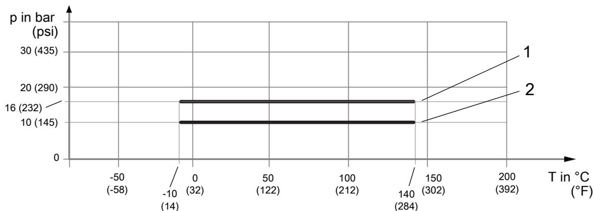
Fig. 9: Allowed process pressure as a function of process fluid temperature
