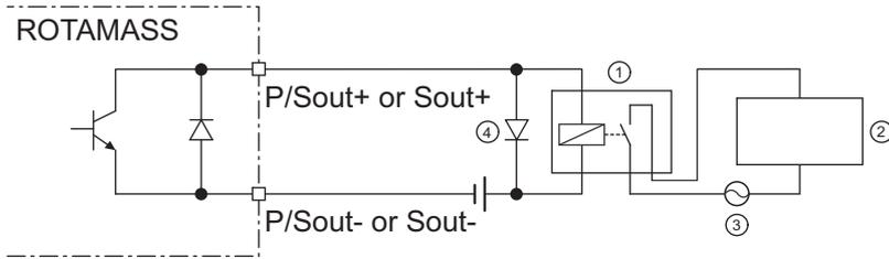
Fig. 33: Passive status output connection *P/Sout* or *Sout* for solenoid valve circuit
