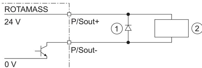
Fig. 26: Active pulse output *P/Sout* connection with electromechanical counter
