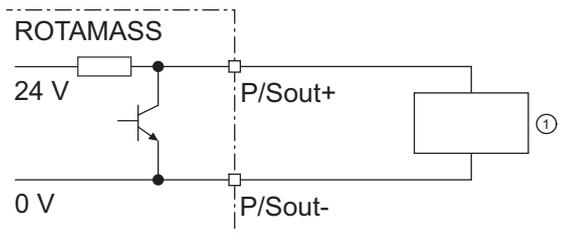
Fig. 31: Active status output P/Sout with internal pull-up resistor
