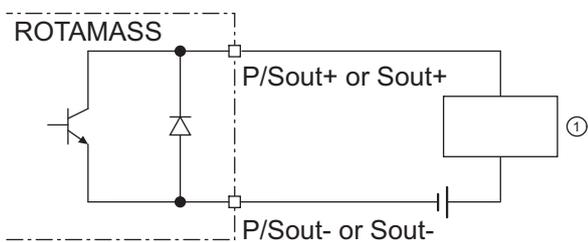
Fig. 32: Passive status output connection P/Sout or Sout
