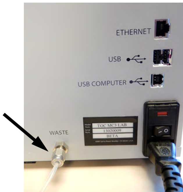
Figure 22: Waste Outlet Fitting — Laboratory TOC Analyzer
