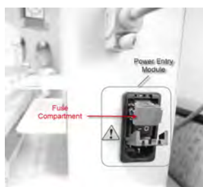
Figure 64: Power Entry Component with Fuse Compartment
