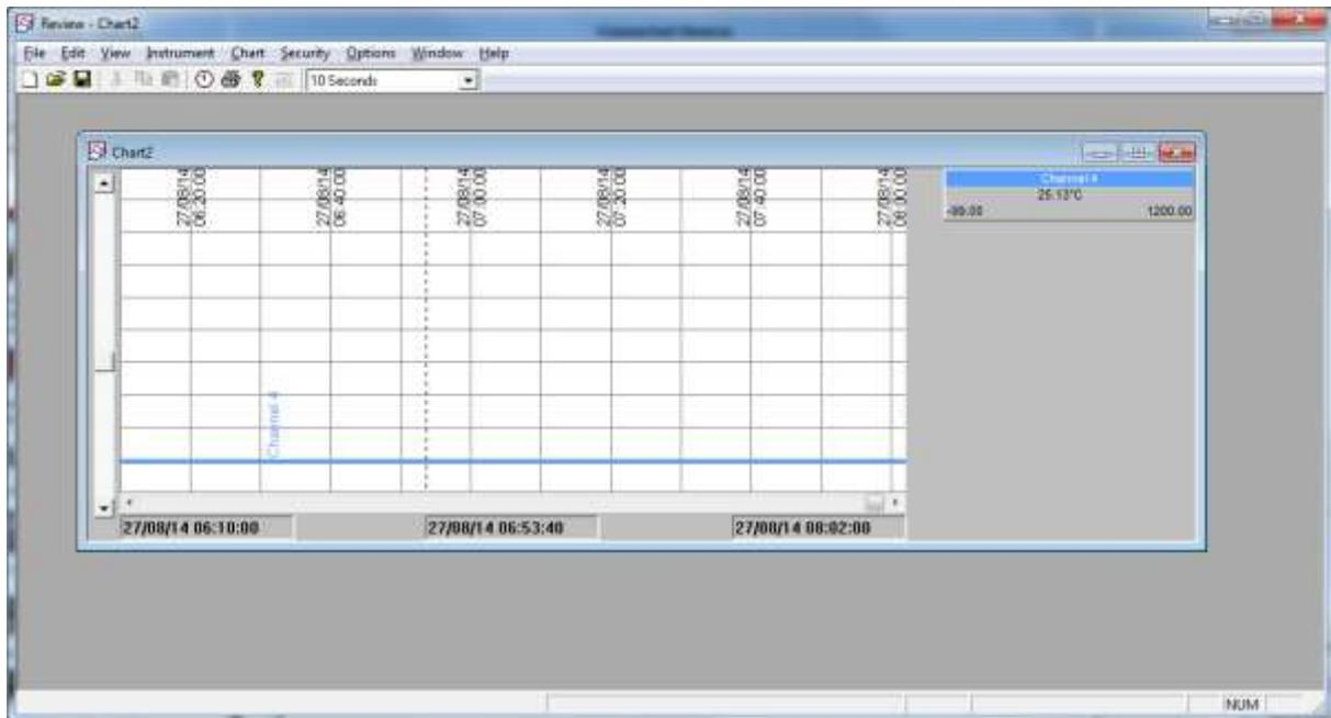
As described in the Review help system, 'Review' allows the user to set up a regular transfer of data (using ftp) from connected instruments into a database on the pc, and then from this database to the chart or spreadsheet. The chart/spreadsheet can be configured to include one or more 'channels' from one or all connected instruments.
