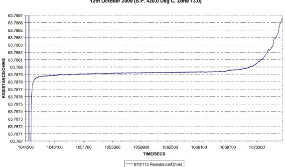
Isothermal Tower Zinc Fixed Point Cell MELT PLATEAU 12th October 2009 (S.P. 420.0 Deg C, Zone 13.0)
