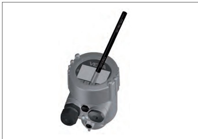
Fig. 26: Display and adjustment module - with adjustment via magnetic pen
