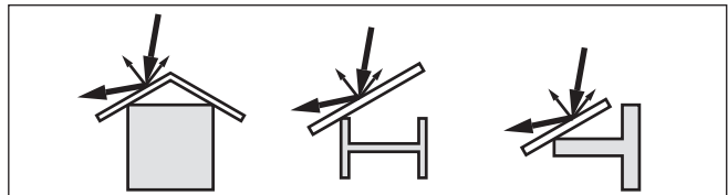
Fig. 12: Cover flat, large-area profiles with deflectors
