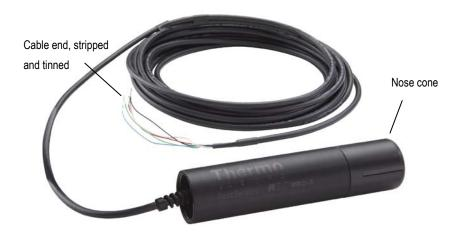
The System is used for continuous monitoring of dissolved oxygen from 0 ppm to 20 ppm. The system also measures temperature from 0°C to 100°C. The optical sensor head is precalibrated and the zero is factory set. The sensor retains calibration values and does not require a new calibration when the system is connected to a new AV38 Display Unit, AquaPro, PC, or PLC.
