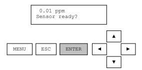
Once the actual zero calibration has been initiated; the display will indicate that a calculation is progressing. During the calculation it is important that nothing disturb the measurement sample. To abort the calibration during this calculation, press ESC.
