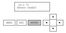
When the sensor is ready, the ENTER key is pressed and the user is presented with a calibration value for editing. Please note that it is best to calibrate temperature when the sensor and the process are at equilibrium.
