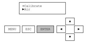
The current sensor value is dynamically displayed and the user is prompted to be sure the measurement is ready for calibration before proceeding. When ready, press the ENTER key.
