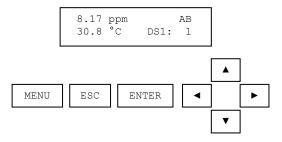
When the RDO Pro-X Optical Dissolved Oxygen System is not connected to the AV38 display, the measure screen indicates the fault as shown in Figure 6.2.
