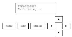
After the calibration point has been stored, the user is prompted to confirm a successful calibration procedure.
