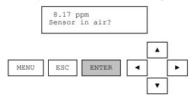
Once the actual air calibration has been initiated; the display will indicate that a calculation is progressing. During the calculation it is important that nothing disturb the measurement sample. To abort the calibration during this calculation, press ESC.
