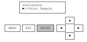
The current sensor value is dynamically displayed and asks the user to be sure the measurement is ready for calibration before proceeding. When ready, press the ENTER key.
