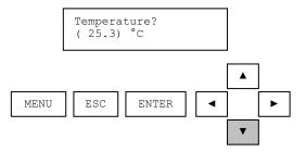
When the value has been edited as desired, the enter key is pressed and the calibration of the point is started.
