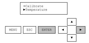
When the temperature calibration procedure is started, the analog output is placed into hold mode. The user is prompted to prepare the sensor. The temperature value is dynamically updated during this step.
