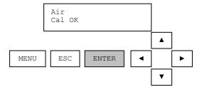
If the calibration is successful, pressing ENTER will return to the measure screen. If the calibration is not successful, pressing ENTER will return to the beginning of the 1-point sample calibration. Reasons for calibration failure include a sample that is not in the correct measurement range or is changing in value too quickly.
