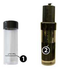
2. Completely submerge the foil of the sensor, making sure that the temperature thermistor is also completely submerged under the surface of the solution. Do not allow the foil to rest completely on the bottom of the calibration chamber. Leave at least 1/2-inch between the surface of the foil and the bottom of the chamber.
