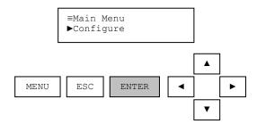
From the Configure menu, use the up/down arrows to select Sensor Filter. Then press ENTER.
