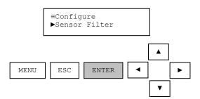
Edit the sensor filter with the up/down arrows. Press ENTER to select a new filter value. Press ESC to abort the new sensor value. The temperature filter edit screen works the same way.
