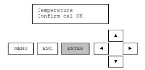
When the enter key is pressed, the analog output is placed into active mode and the monitoring of sensor and temperature values is resumed. This successfully completes the temperature calibration procedure.
