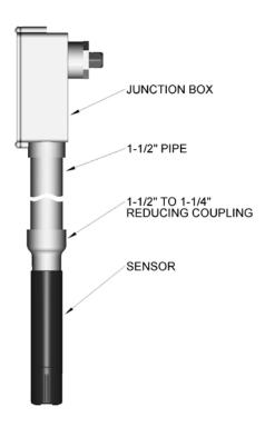
This immersion assembly can be ordered by itself, with a hand rail mounting assembly or with a ball float that keeps the sensor a fixed distance below the surface of the water. Part numbers for the mounting assemblies are shown in the following table.
