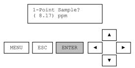
Once the actual 1-point sample calibration has been initiated; the display will indicate that a calculation is progressing. During this calculation it is important that nothing disturb the measurement sample.
