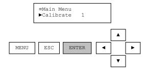
From the Calibrate Menu, use the up/down arrows to select 1-Point Sample. Then press ENTER.
