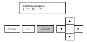
During this time, the calibration procedure can be aborted by pressing the escape key.
