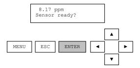
The calibration value can be adjusted with the arrow keys. Use the up/down arrows for fine adjust and the left/right arrows for coarse adjust. After the calibration value is adjusted to the desired value, press the ENTER key.
